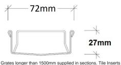
Grates longer than 1500mm supplied in sections. The inserts longer than 1200mm supplied in sections. Channels over 3000mm supplied in sections with joiner. +/-2mm tolerance on dimensions.
