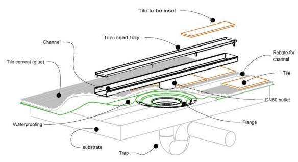
NOTE, this method require the channel system to be ABOVE and SEPARATE from the waterproofing
