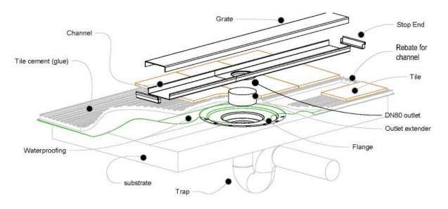
NOTE, this method requires the channel system to be ABOVE and SEPARATE from the WATERPROOFING.
