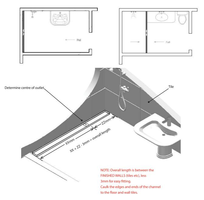
After determining the overall size less 3mm, measure both sides from the centre of the outlet to cut the channel to size.
