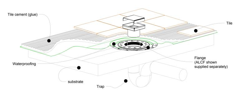
NOTE, this method requires the channel system to be above and separate from the waterproofing
