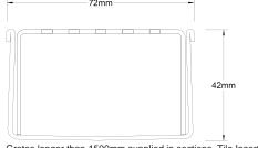
Grates longer than 1500mm supplied in sections. Tile Inserts longer than 1200mm supplied in sections. Channels over 3000mm supplied in sections with joiner. +/-2mm tolerance on dimensions.
