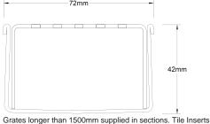
Grates longer than 1500mm supplied in sections. The inserts longer than 1200mm supplied in sections. Channels over 3000mm supplied in sections with joiner. +/-2mm tolerance on dimensions.
