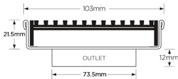
Grates longer than 1500mm supplied in sections. Tile Inserts longer than 1200mm supplied in sections. Channels over 3000mm supplied in sections with joiner. +/-2mm tolerance on dimensions.
