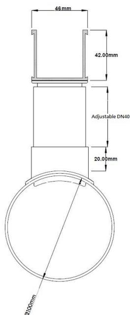
Grates longer than 1500mm supplied in sections. Tile Inserts longer than 1200mm supplied in sections. Channels over 3000mm supplied in sections with joiner. +/-2mm tolerance on dimensions.
