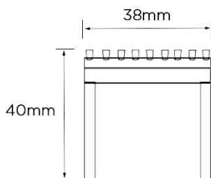
Grates longer than 1500mm supplied in sections. Tile Inserts longer than 1200mm supplied in sections. Channels over 3000mm supplied in sections with joiner. +/-2mm tolerance on dimensions.
