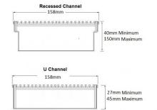
Grates longer than 1500mm supplied in sections. Tile Inserts longer than 1200mm supplied in sections. Channels over 3000mm supplied in sections with joiner. +/-2mm tolerance on dimensions.
