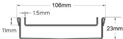
Grates longer than 1500mm supplied in sections. Tile Inserts longer than 1200mm supplied in sections. Channels over 3000mm supplied in sections with joiner. +/-2mm tolerance on dimensions.
