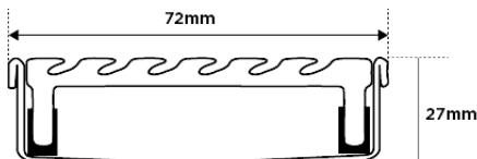
Grates longer than 1500mm supplied in sections. Tile Inserts longer than 1200mm supplied in sections. Channels over 3000mm supplied in sections with joiner. +/-2mm tolerance on dimensions.
