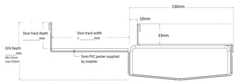
SQ100Ti33DN80 floor wastes to sit above each outlet. Floor waste suits up to a 25mm tile/ stone.
