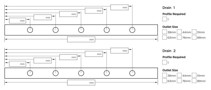
**NOTE:** See AS3500 standard & local regulator for specific outlet/drain requirements. Outlet Size must be smaller than selected Range. MND grate style not available with Profiles 2 or 4. Stainless Steel Grade is 316 unless specified. Made-to-Length (MTL) minimum charge of 800mm. Grates over 1500mm are supplied in multiple sections. Channels over 3000mm are supplied in multiple sections with joiner. Orders received after 11am are processed next working day. +/- 2mm tolerance on dimensions.
