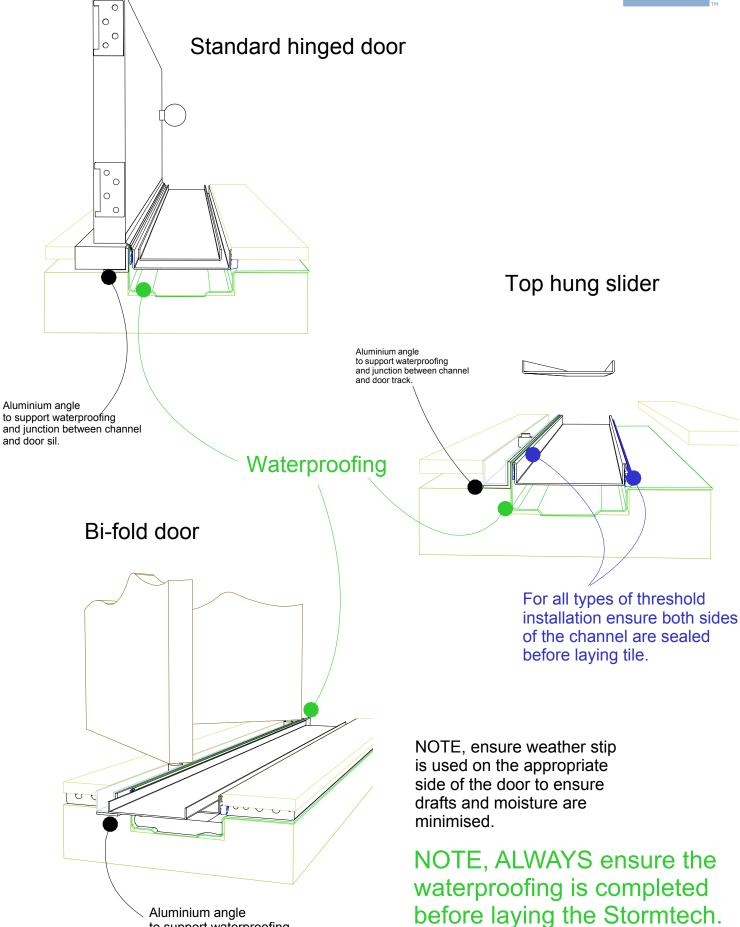
Aluminium angle to support waterproofing and junction between channel
