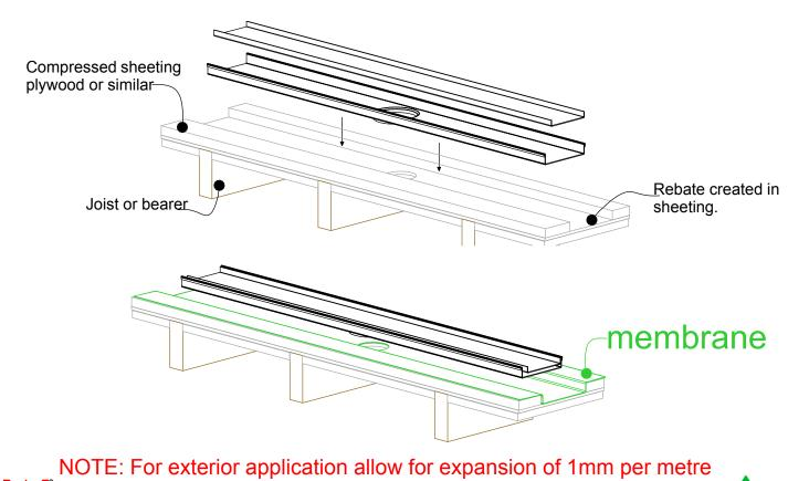
by using quality suitable flexible sealant on channel joins.
