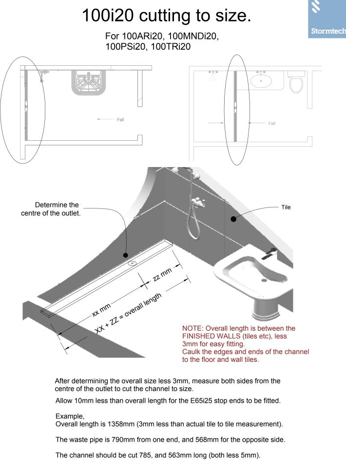
Once the E65i25 stop ends are on and sealed, the overall length will be 1358mm and the outlet will be in the correct position.
