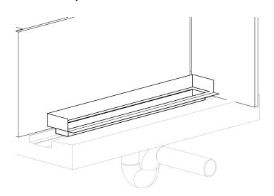
Apply a suitable waterproofing membrane as per relevant standards and building code. The flanged tray is suitable for use as a waterproofing flange.
