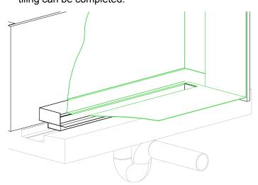
For tiling, ensure the grate is removable and not locked in by tiles.
