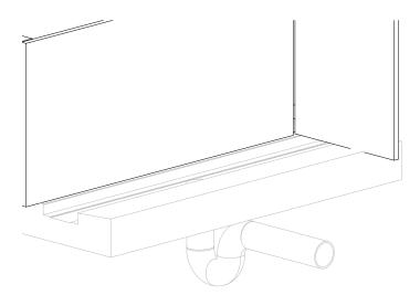
Lay the tray in position with outlet connecting to the riser of the waste.
