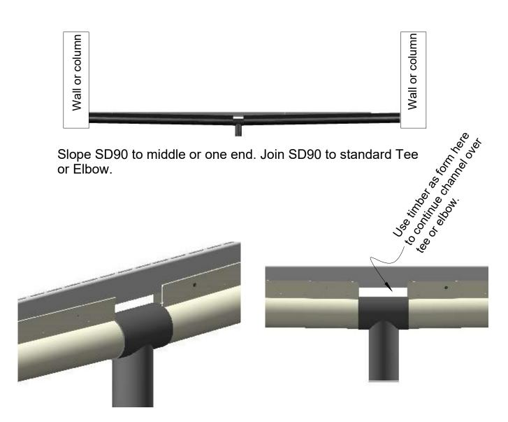
Trim SD90 channel section back from pipe section and use timber to form channel over standard tee or elbow.
